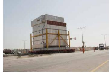
Overall the load measured 14.97 x 14.07 x 17.70 metres (L x W x H), including the height of the trailer, which presented significant logistical challenges. Two 18-axle lines were used side by side to carry the boiler. The first step was to bypass port's 13-metre high conveyor belt by partially removing fencing and the port gate. The second challenge was to avoid the 11-metre high 380 KVA Marafiq power lines, which could not be turned off because it would disrupt Marafig's water production.
